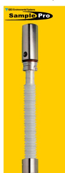
The SamplePro Portable MicroPurge Pump uses a quick-change, one-piece bladder design. Compressed gas squeezes the outside of the bladder to force liquid out of the pump; there is no gas contact with the pumped water inside the bladder.
